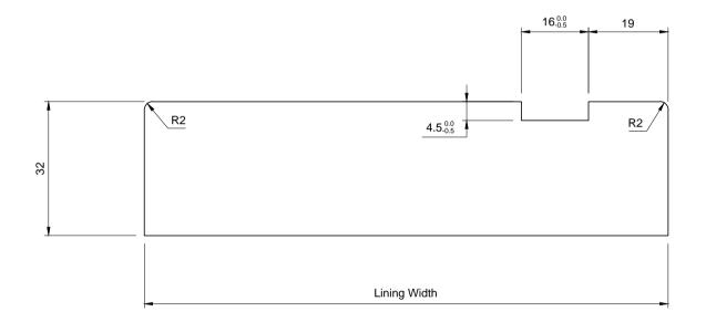
Description: Machining Profile - 32mm Timber Lining - Non Q2F - FD30 - 54mm Core
